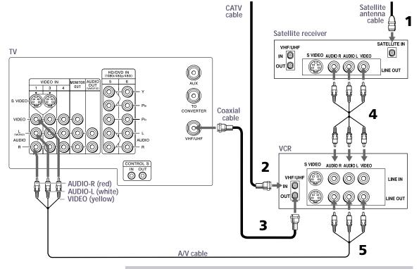
If the peripherals you are connecting have S VIDEO jacks, you can use S VIDEO cables for improved picture quality (compared to combination audio/video cables). Because S VIDEO cables carry only the video signal, you will need audio cables for sound.
